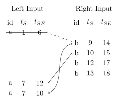
Here, the later element on the left is joined with "not-the-newest" element on the right, even though the element size on the right is set to one. Here we can see, that the elements on the left are joined with the newest possible element of the other side.
