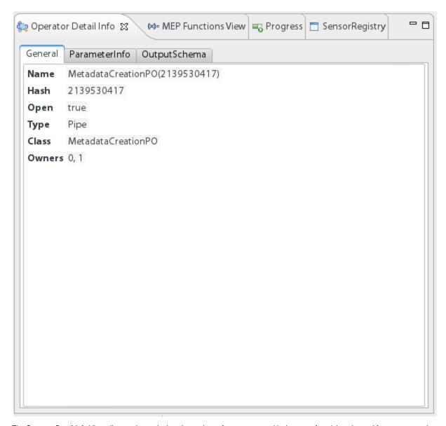
The Operator Detail Info View allows a deeper look to the settings of an operator and is thus a perfect debugging tool for your processing queries.
