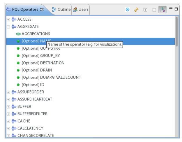
In the PQL Operators View you can see all available PQL Operators including their required and optional parameters. Further, you can get a description of each parameter by moving the mouse over it.
