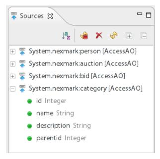
The Sources View contains a list of available sources with their given name and schema information to be used in you processing query. Every time a new source is registered in Odysseus, a new source will be inserted in the list of available sources.
