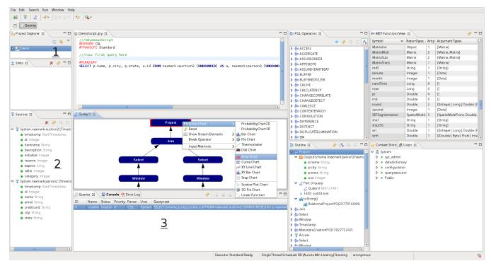
After the login process, the Odysseus RCP GUI starts up. In this GUI you can create a new Odysseus project by issuing a click with the right mouse button in area 1. When you have created a new project you can start creating Queries for your project using any soure listet in area 2 or creating own sources. You can start an Odysseus Query by a click on the Play-Button in the toolbar. All running queries are listet in area 3.
