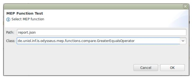
The result of the MEP function test is stored in JSON format and includes a detailed report about all tests including parameter type, value, and stacktrace in case of an error.
